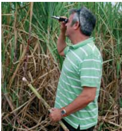
Richard Livermore (Right) using a portable refractometer which measures the amount of pure sucrose in the cane juice.
